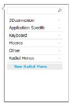
This brings up the Radial Menu Editor where you can assign a name and commands to the different sections. Your new Radial Menu will be automatically assigned to the button from where you opened the panel. Enabling "Gestures" allows commands mapped to the radial menu to be executed by moving the cursor past the desired command, without having to click the radial menu button.
