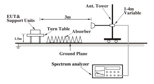
Note: For the actual test configuration, please refer to the attached file (Test Setup Photo).
