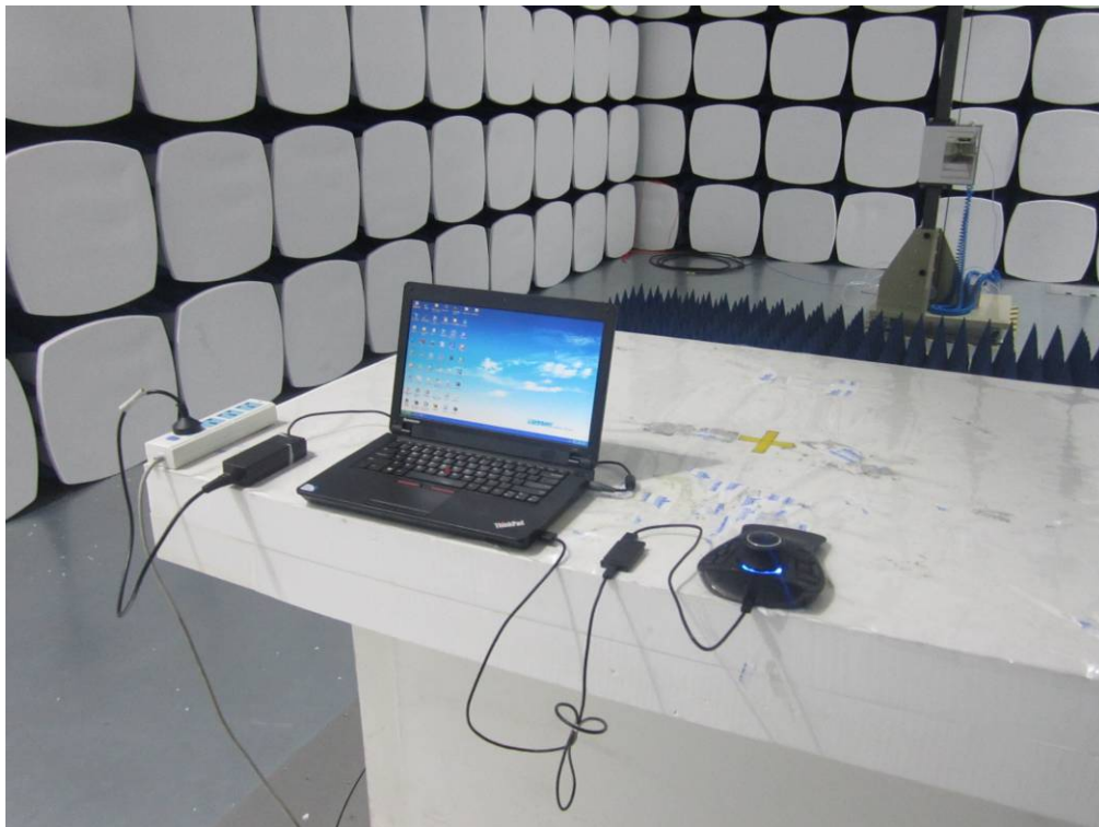
Radiated Spurious Emissions Test Setup Above 1GHz –Front View (3Dconnexion USB HUB(Model:3DX-600049) has been tested)
