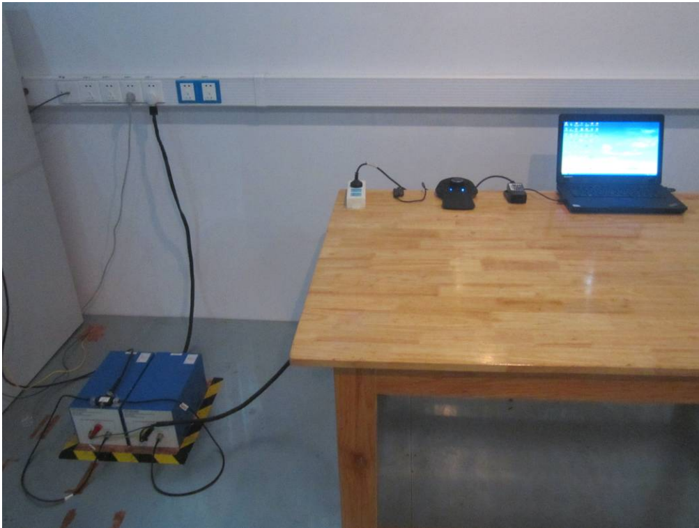
Conducted Emissions Test Setup Front View (3Dconnexion USB HUB(Model:3DX-600049) has been tested)
