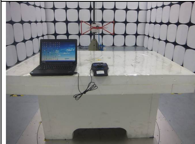
Radiated Emissions Test Setup Below 1GHz
