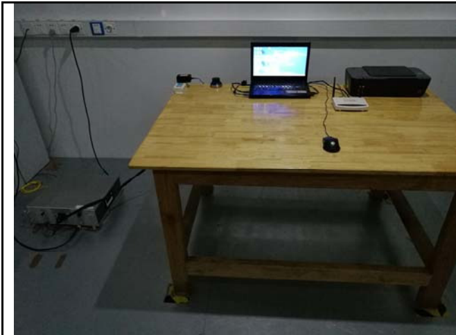
Conducted Emissions Test Setup – Front View
