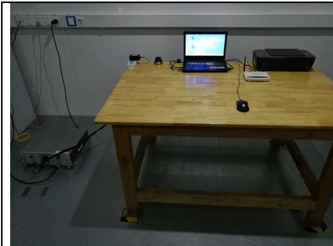
Conducted Emissions Test Setup – Front View
