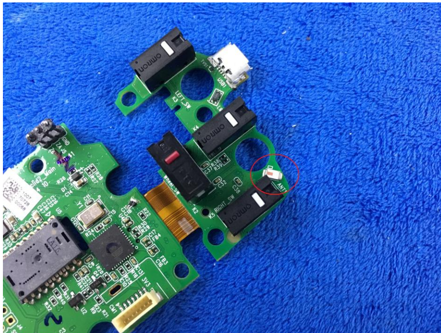
BT - Antenna View
