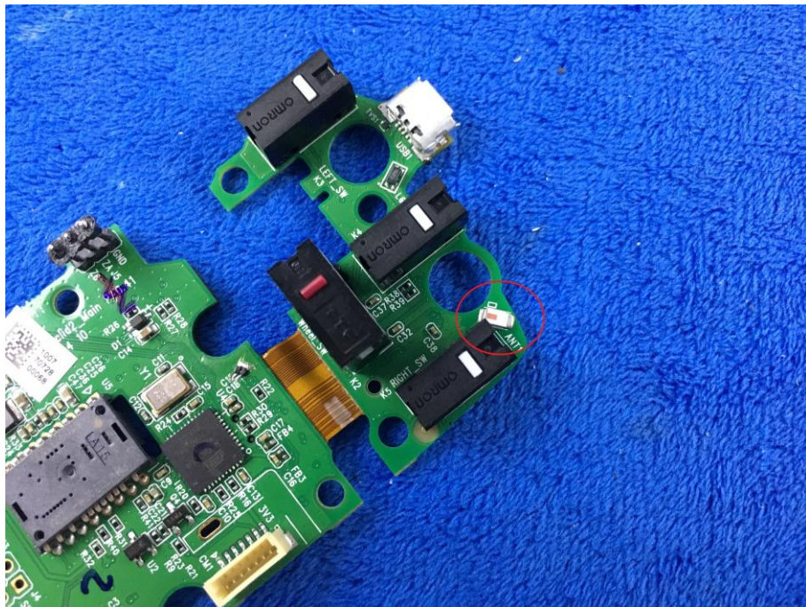
BT - Antenna View
