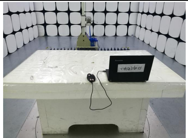
Radiated Emissions Test Setup Above 1GHz
