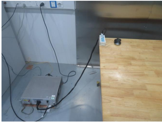
Conducted Emissions Test Setup Front View
