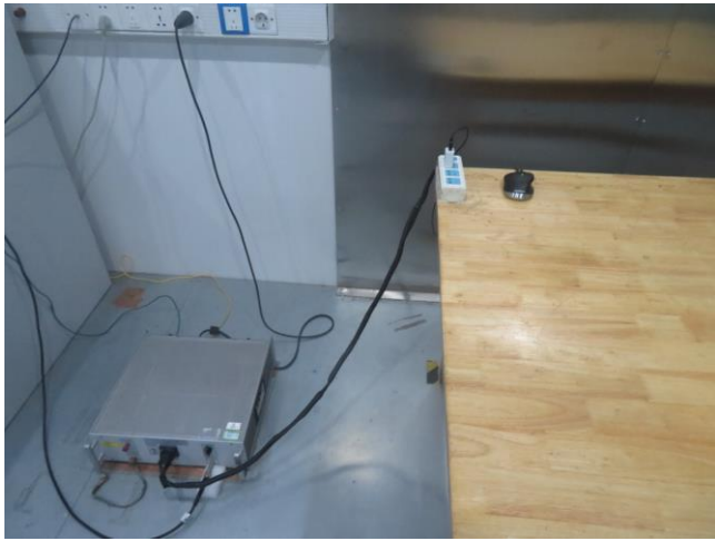
Conducted Emissions Test Setup Front View
