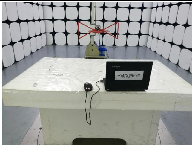
Radiated Emissions Test Setup Below 1GHz
