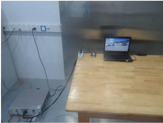
Conducted Emissions Test Setup Front View
