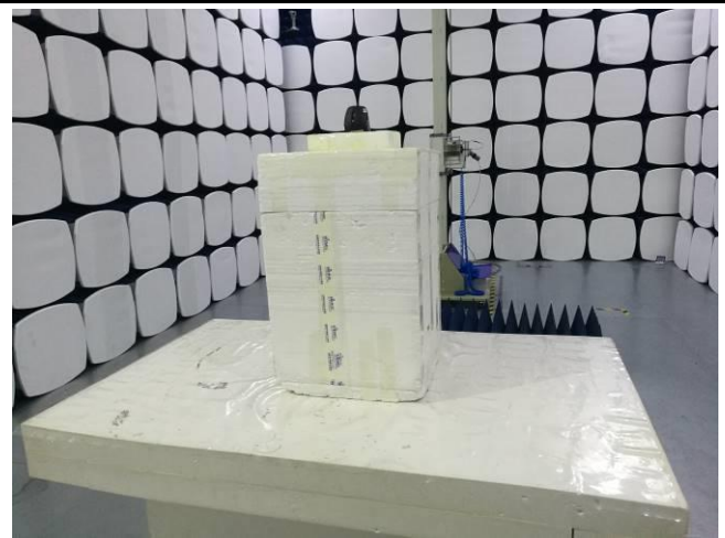
Radiated Spurious Emissions Test Setup Above 1GHz
