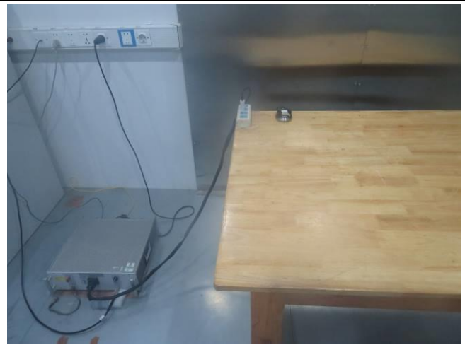
Conducted Emissions Test Setup Side View
