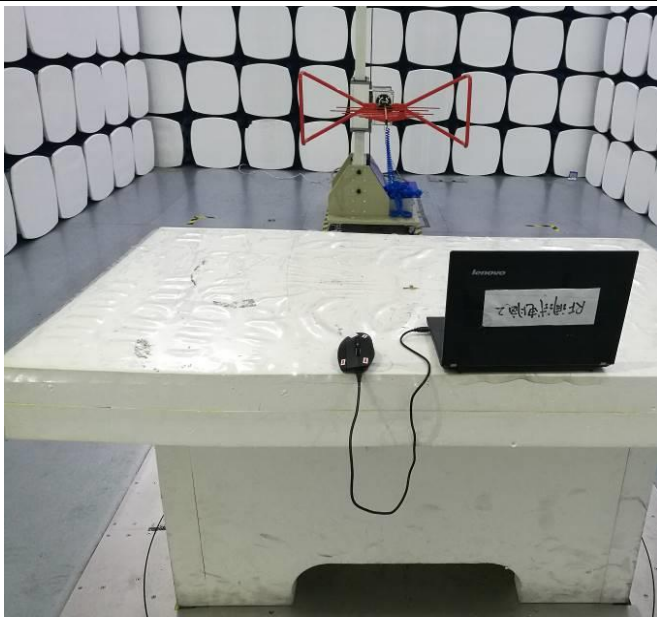
Radiated Emissions Test Setup Below 1GHz
