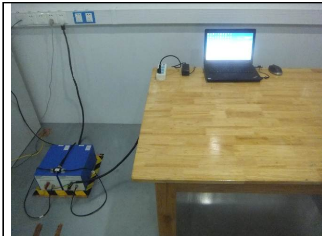
Conducted Emissions Test Setup – Front View
