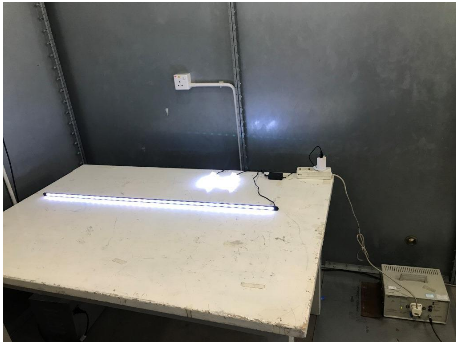
Measurement of Conducted Emission Test Set Up
