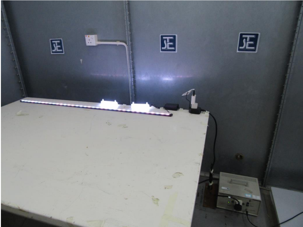
Measurement of Conducted Emission Test Set Up
