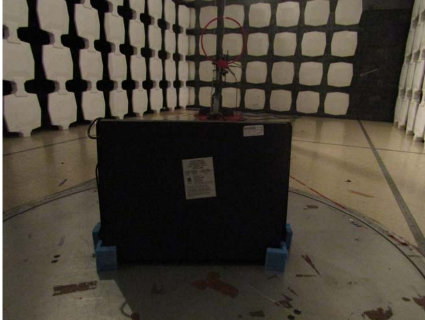
Measurement of Radiated Emission Test Set Up (9kHz to 30MHz)
