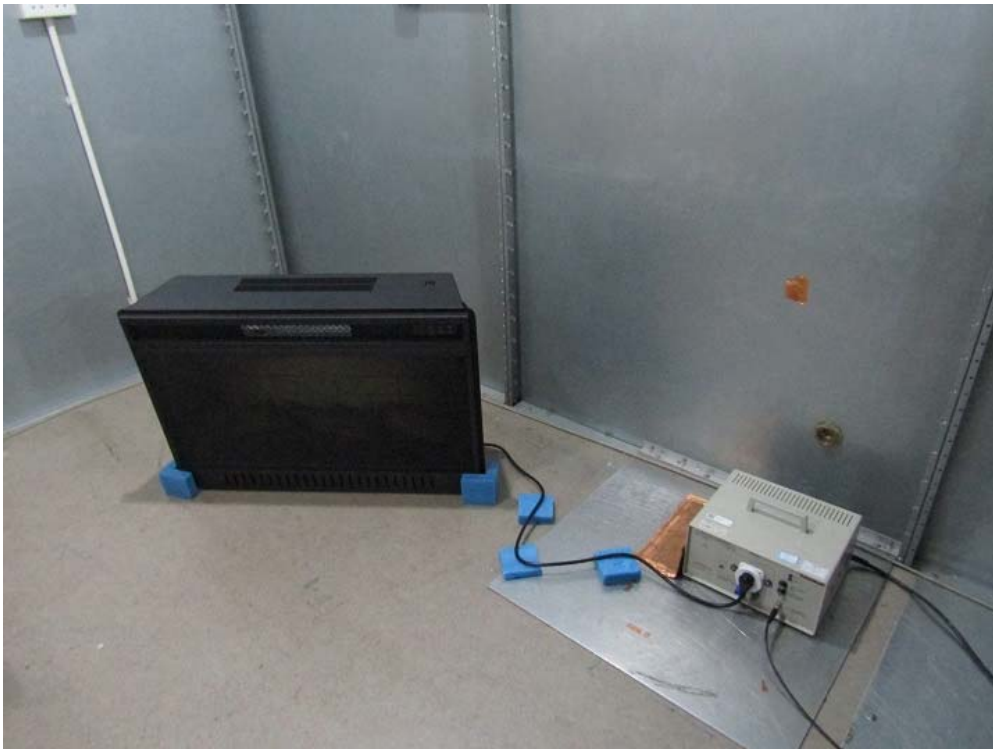
Measurement of Conducted Emission Test Set Up
