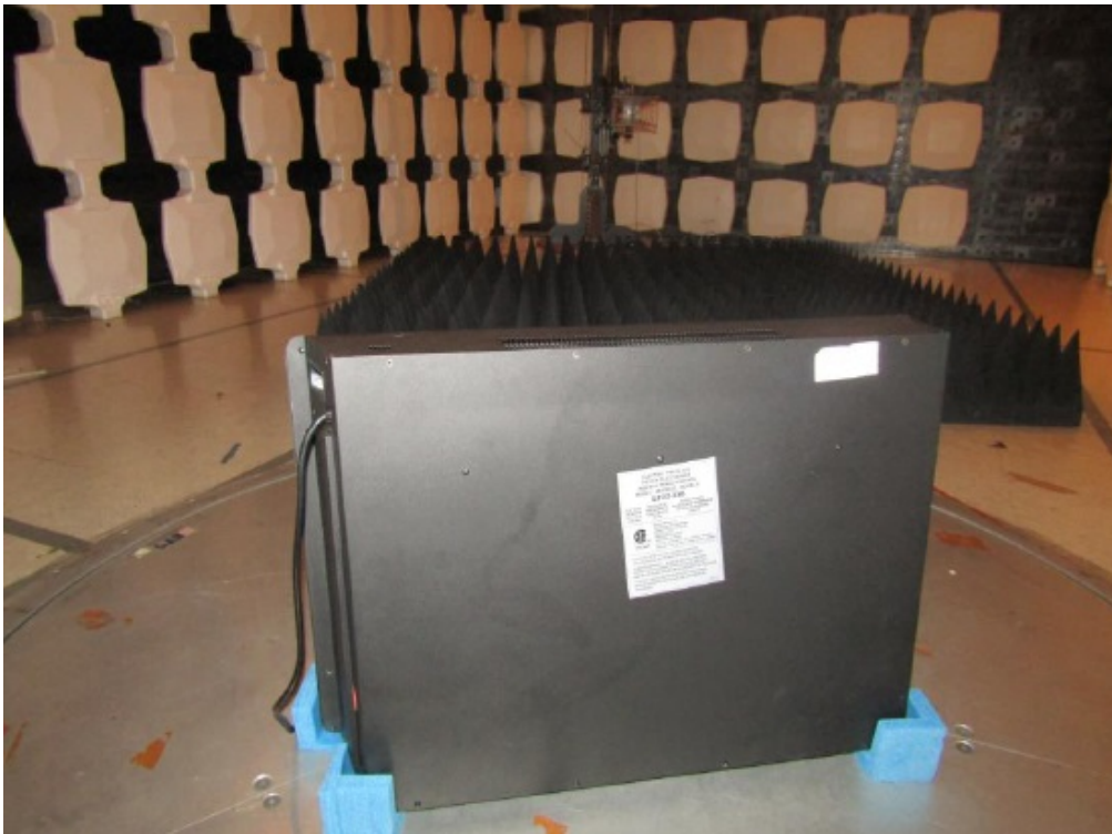
Measurement of Radiated Emission Test Set Up
