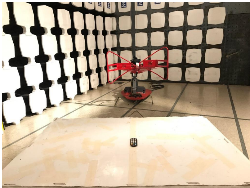
Measurement of Radiated Emission Test Set Up
