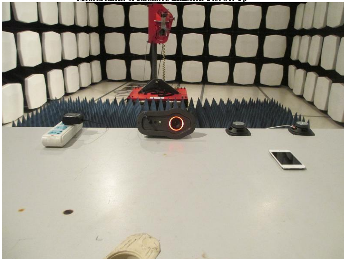
Measurement of Radiated Emission Test Set Up
