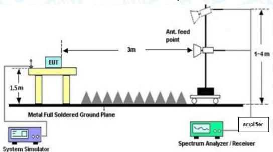
**Above 1GHz Test Setup**
