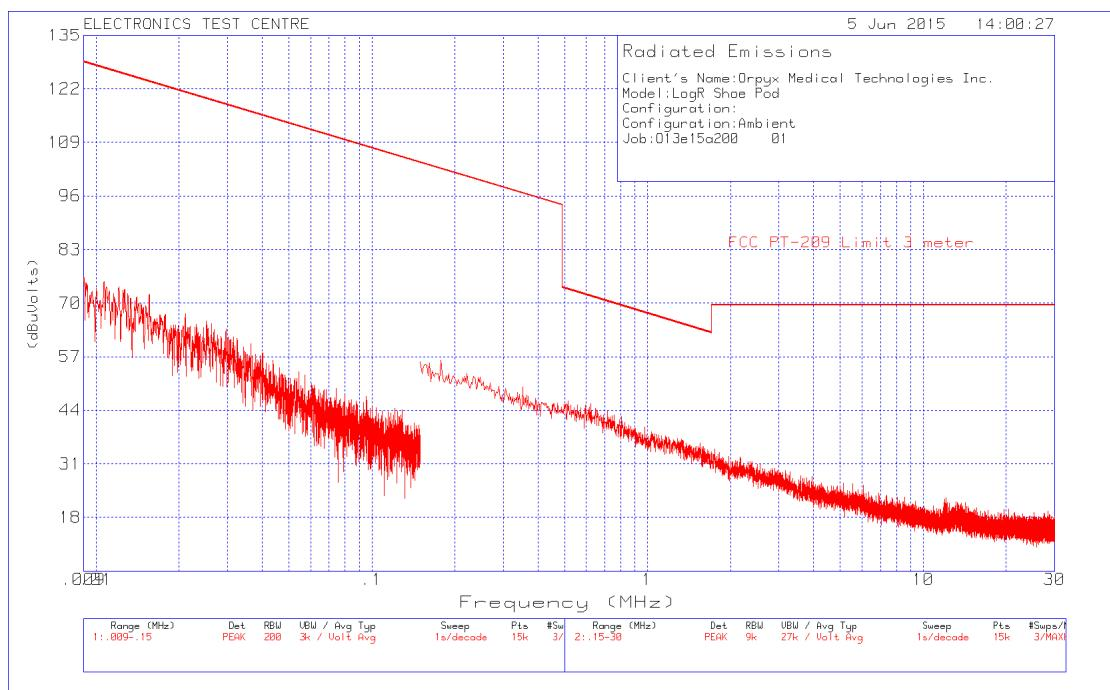
**aPlot of Test Chamber Ambient: (measurement noise floor):**
