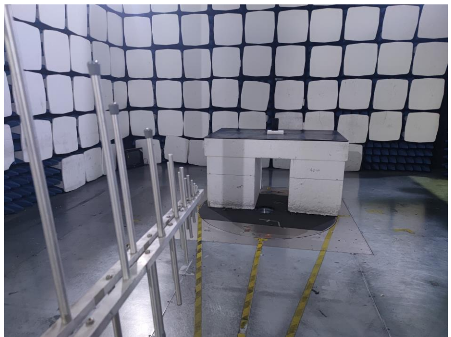
Radiation Emission Test Setup (30MHz to1GHz)
