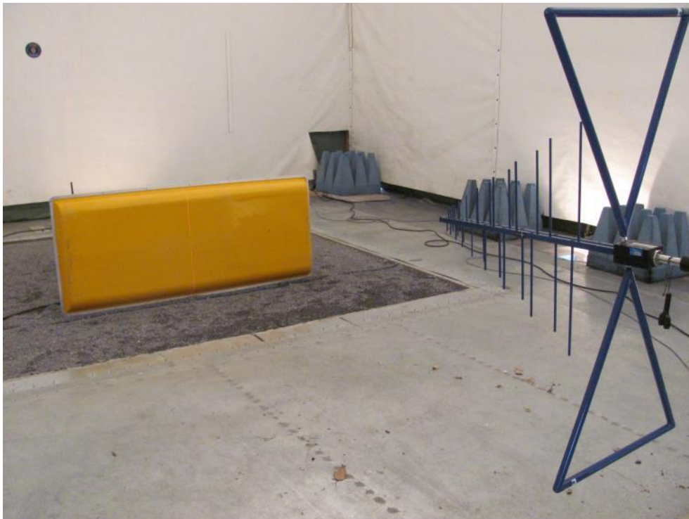
Picture 5. Measurement setup, 30 MHz – 1 GHz.
