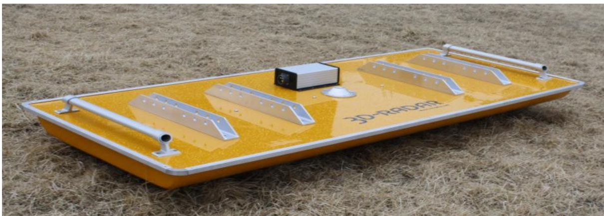
Figure 5. DXG antenna completely assembled with top cover.
