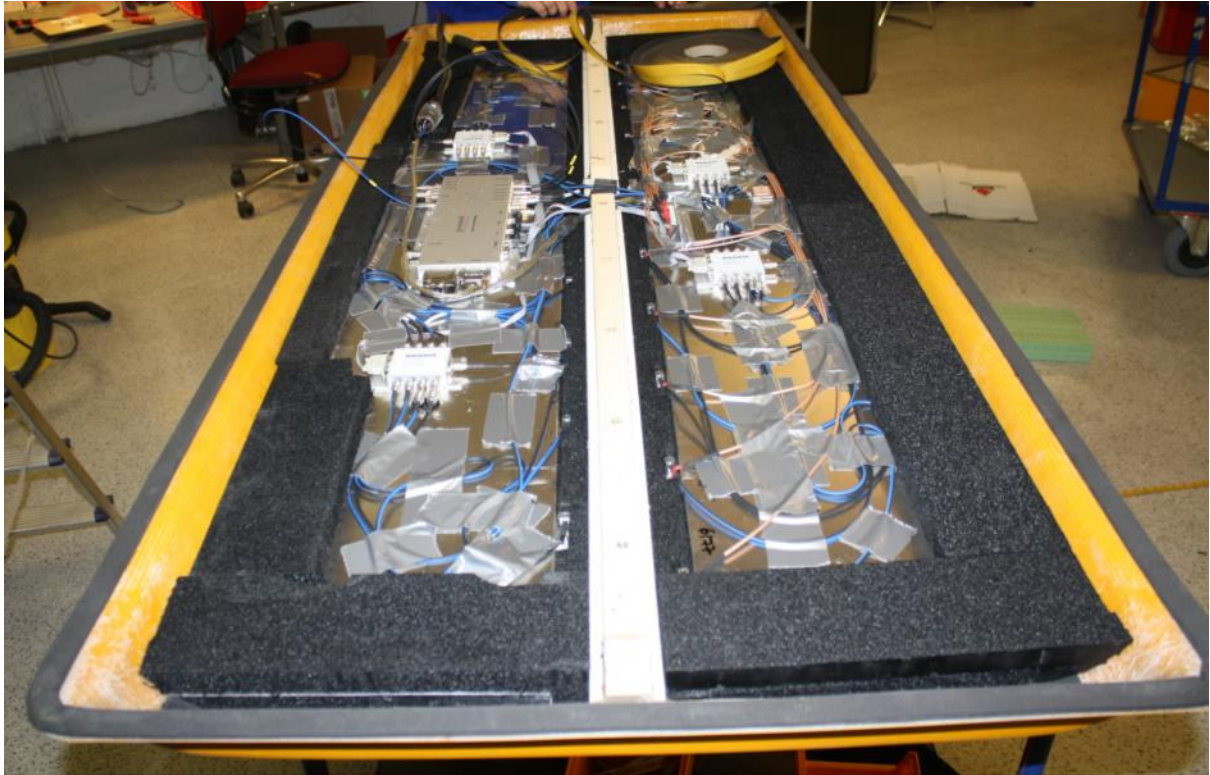
Figure 4. DXG antenna without top cover. Microwave absorbers are located on the top side of the ground plane.
