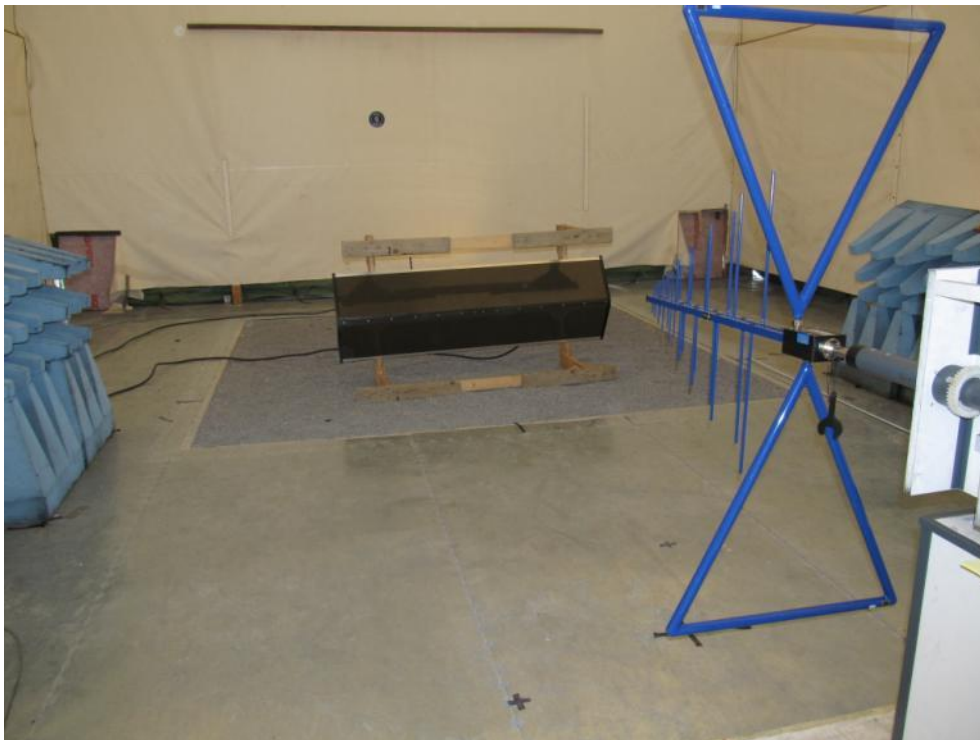
Picture 5. Measurement setup, 30 MHz – 1 GHz.
