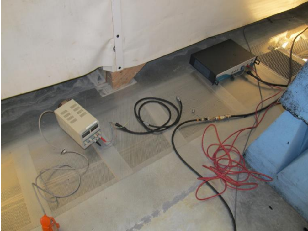
Picture 2. The GeoScope with its power supply unit placed beside the test area.
