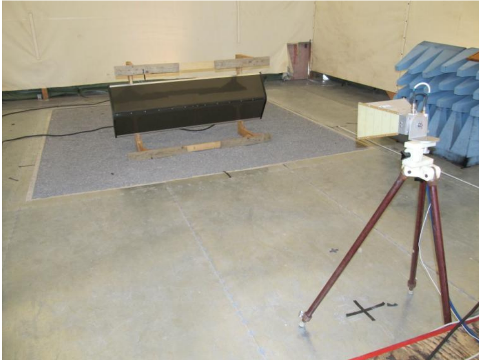
Picture 6. Measurement setup, 1 GHz – 4 GHz.
