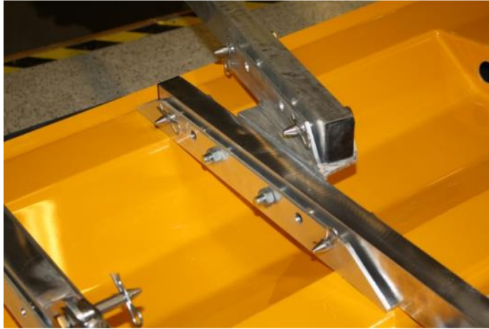
Figure 14 – Installation of tow bars.
