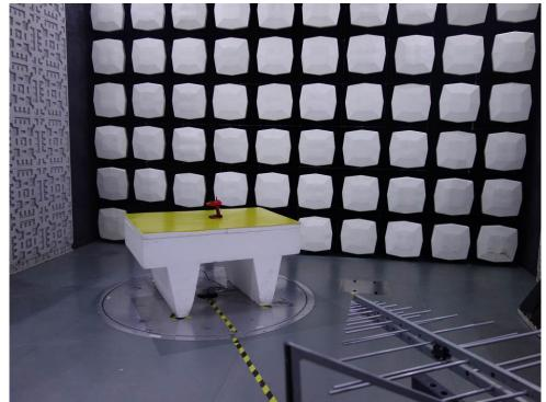
8.2 Radiated Emissions Test Setup (Above 1GHz)
