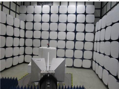
8.3 Restricted Band Around Fundamental Frequency Test setup
