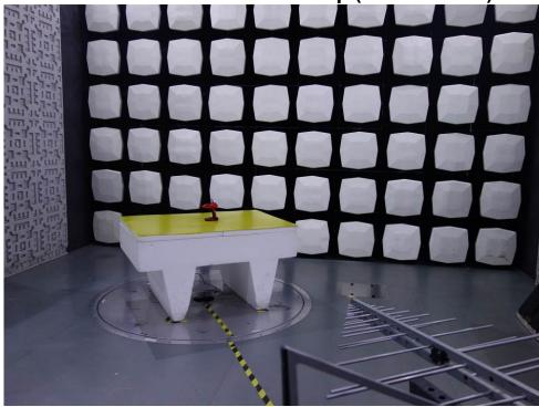
1.2 Radiated Emissions Test Setup (Above 1GHz)
