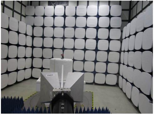
1.4 Field Strength of the Fundamental Signal (15.249(a)) Test Setup
