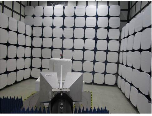
1.3 Restricted Band Around Fundamental Frequency Test setup
