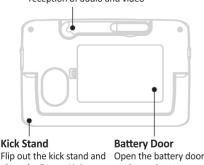
place the Parent Unit on a stable, level surface.
