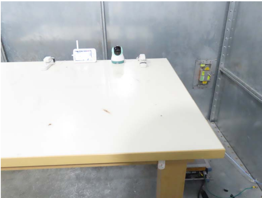
Set Up Photo of Conducted Emission
