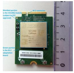
The VZ120Q can be used on the M.2 adaptation board plugged into an evaluation kit that provides standard easily accessible interfaces, e.g. USB and UART (debug) connectivity, SIM access, or antenna connection... as depicted below. That's the test board which is used below in section 2.
