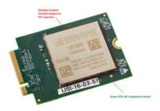
The US130Q can be used on the M.2 adaptation board plugged into an evaluation kit that provides standard easily accessible interfaces, e.g. USB and UART (debug) connectivity, SIM access, or antenna connection... as depicted below. That's the test board which is used below in section 2.
