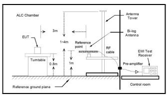
Radiated measurements > 1GHz
