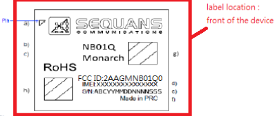
Figure 3-6: NB01Q-0 Marking Description
