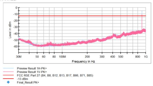
The peak above the limit is the LTE Cat. M1 Band 106 carrier frequency.
