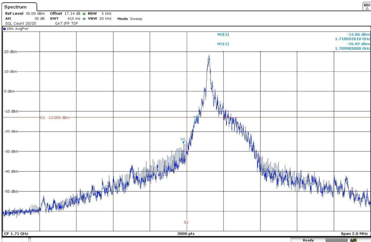
12 Tones 15 kHz, Offset Tone = 0.  $\pi/4$  - QPSK modulation. Low Block Edge:
