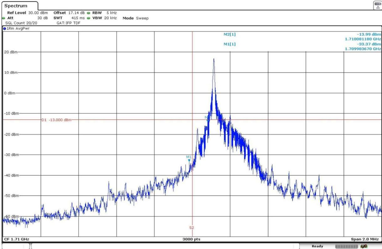
1 Tone 15 kHz, Offset Tone = 0.  $\pi/4$  - QPSK modulation. Low Block Edge:
