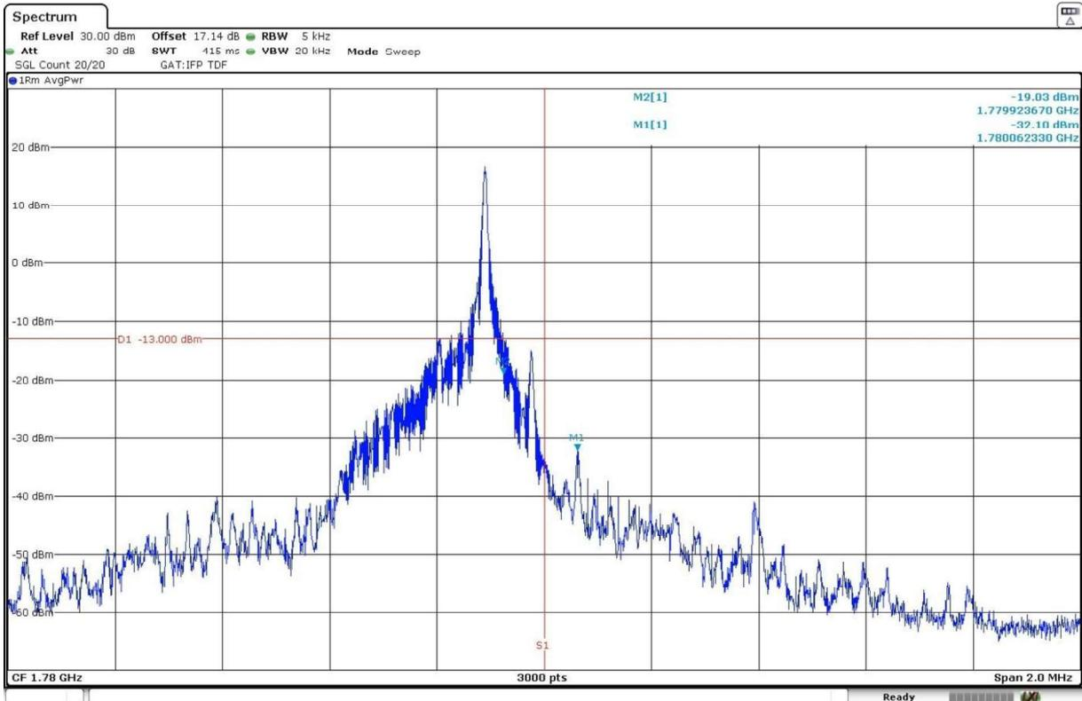
1 Tone 15 kHz, Offset Tone =  $11 \cdot \pi/4$  - QPSK modulation. High Block Edge:
