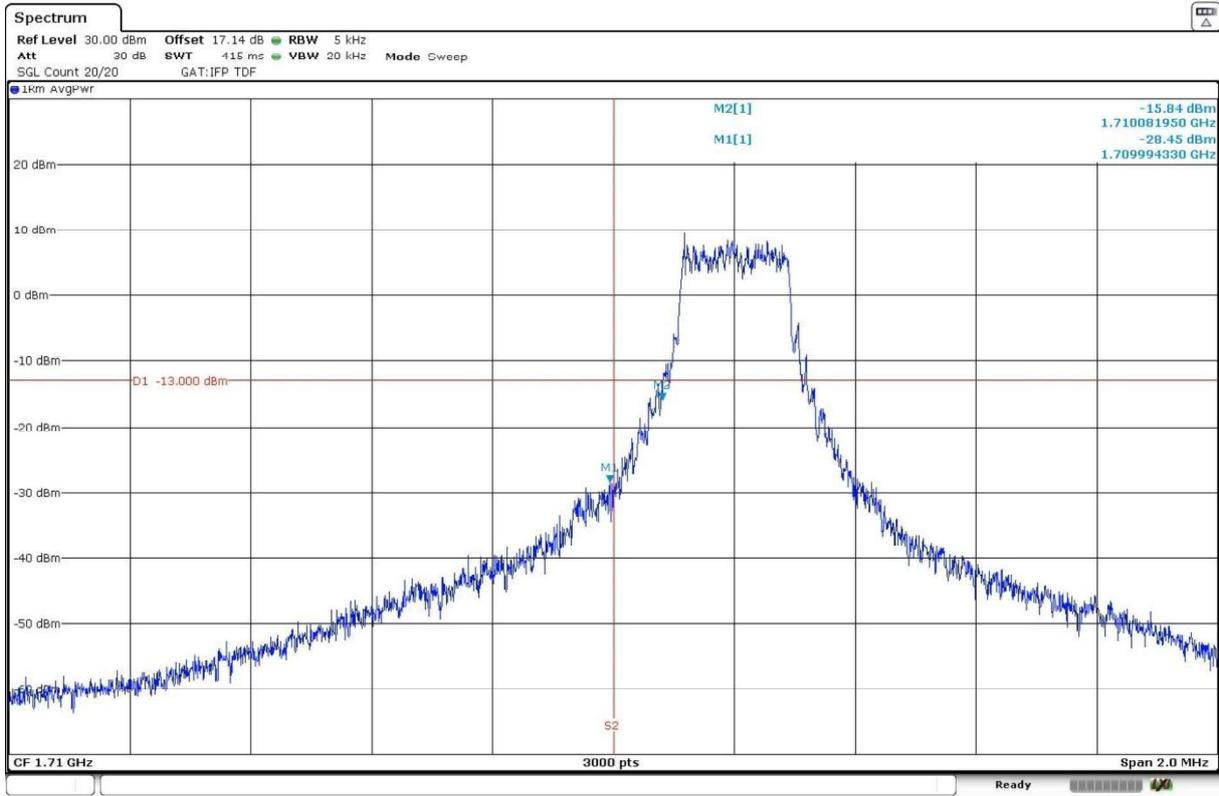
1 Tone 3.75 kHz, Offset Tone = 47.  $\pi/4$  - QPSK modulation. High Block Edge:
