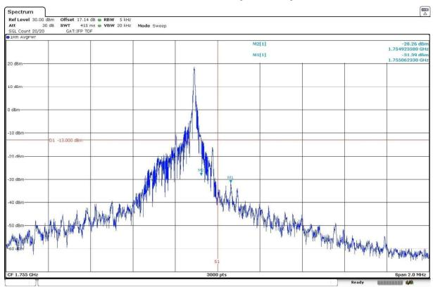
1 Tone 15 kHz, Offset Tone = 11.  $\pi/4$  - QPSK modulation. High Block Edge:
