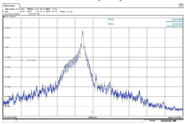
12 Tones 15 kHz, Offset Tone = 0.  $\pi/4$  - QPSK modulation. High Block Edge:
