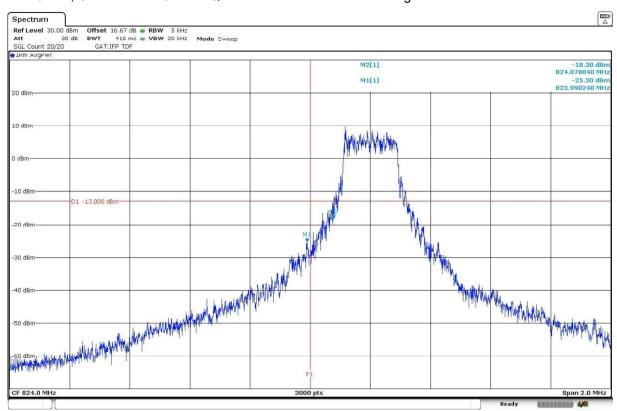
1 Tone 3.75 kHz, Offset Tone = 47.  $\pi/4$  - QPSK modulation. High Block Edge:
