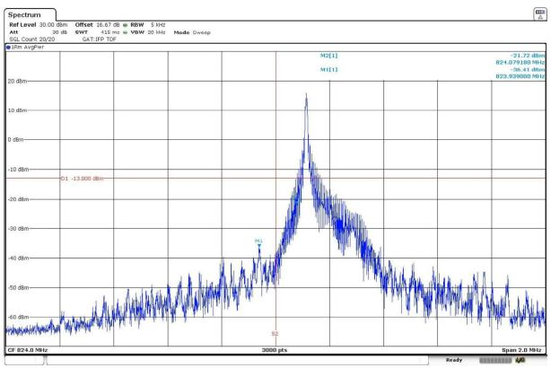
1 Tone 15 kHz, Offset Tone = 0.  $\pi/2$  – BPSK modulation. Low Block Edge:
