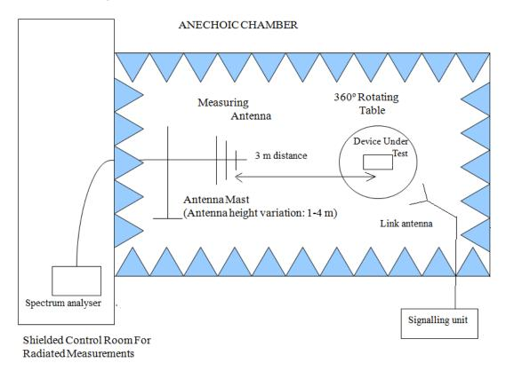
Radiated measurements setup from 1 GHz to 18 GHz:
