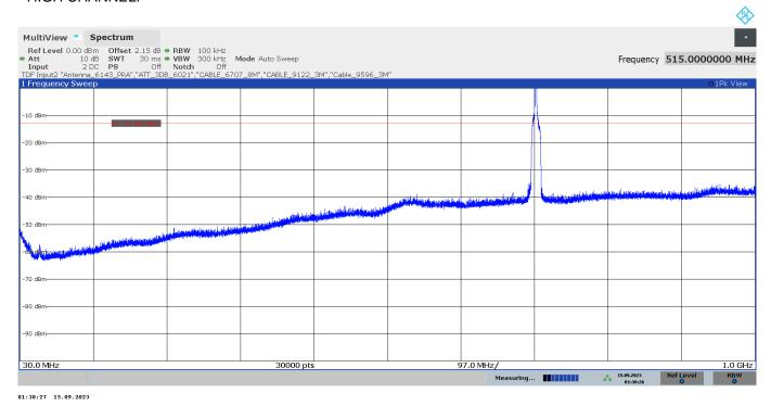
The peak above the limit is the LTE Cat 1bis Band 12 carrier frequency.
