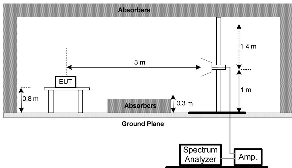
**(C) Radiated emissions below 30MHz**
