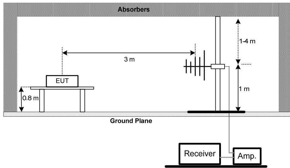
**(B) Radiated Emission Test Set-Up Frequency Above 1 GHz**
