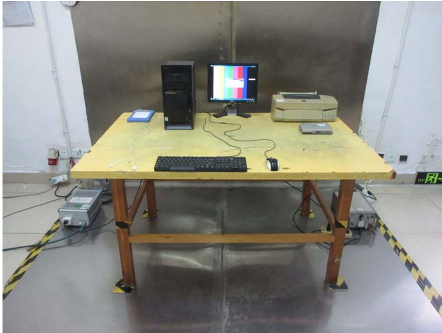
Conducted Emission Test Setup Front View
