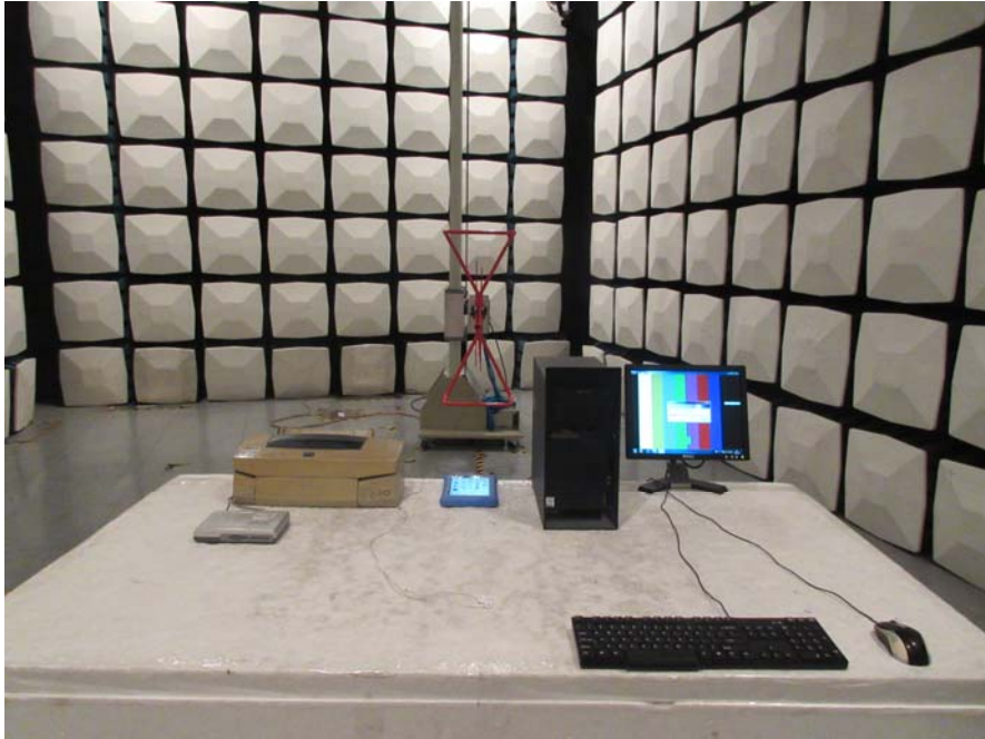
Radiated Disturbance Test Setup Rear View (Below 1GHz)
