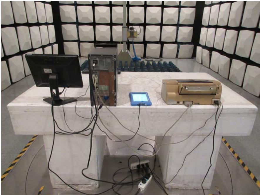
Radiated Disturbance Test Setup Rear View (Above 1GHz)
