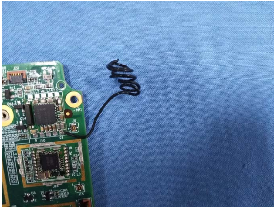
EUT – FM Antenna View
