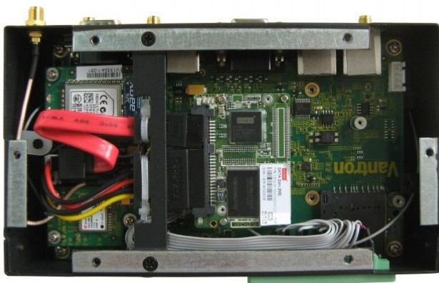
Bottom View for optional embedded modules (1xHalf PCIe slot under the 1xPCIe slot)
