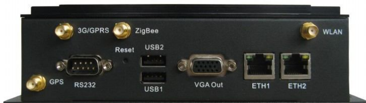
3G / GPRS Antenna(3G Band) Antenna Gain:1dBi
