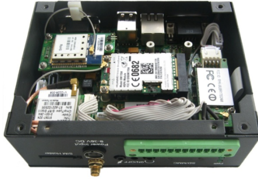
Bottom View for optional embedded modules (1xHalf PCIe slot under the 1xPCIe slot)
