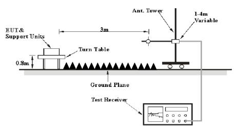
The radiated emission tests were performed in the 3 meters chamber test site, using the setup accordance with the ANSI C63.4-2003. The specification used was the FCC 15.209, and FCC 15.247 limits. The external I/O cables were draped along the test table and formed a bundle 30 to 40 cm long in the middle.
