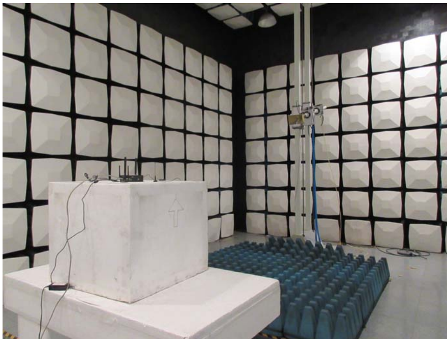
Radiated Emissions Test Setup View (Above 1GHz)
