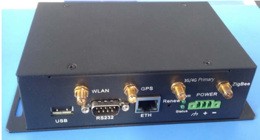
EUT – Front Port View
