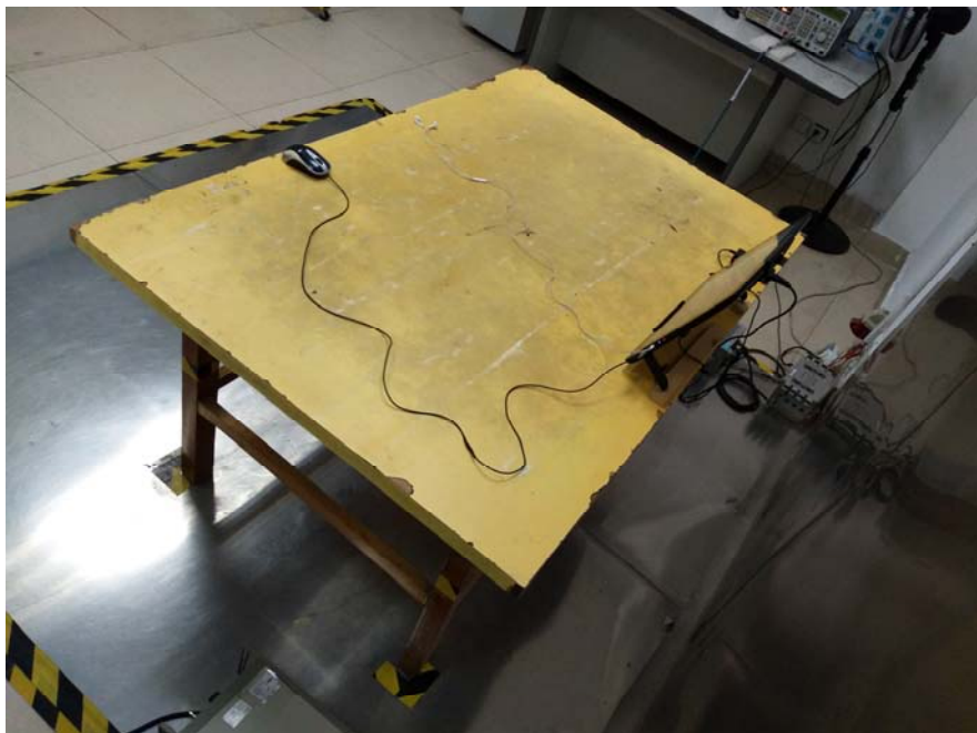
Conducted Emission Test Setup Side View
