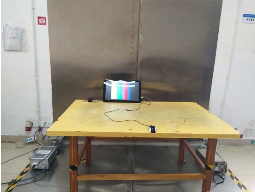
Conducted Emission Test Setup Side View
