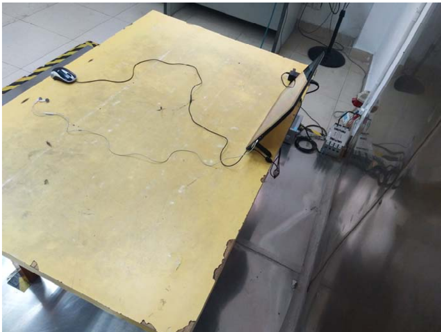
Conducted Emission Test Setup Side View
