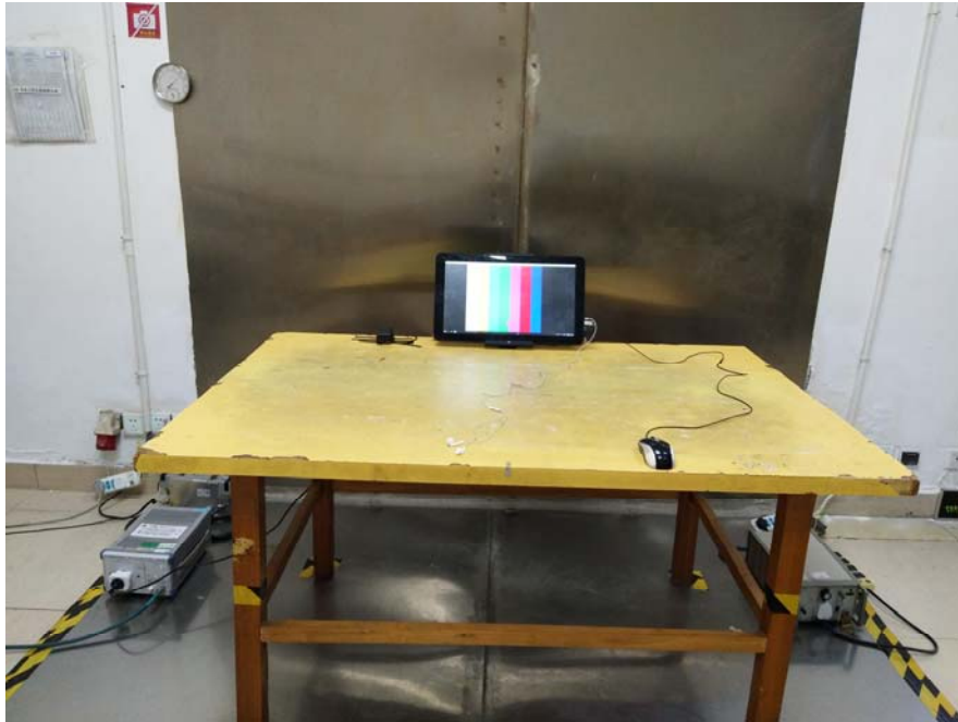
Conducted Emission Test Setup Side View
