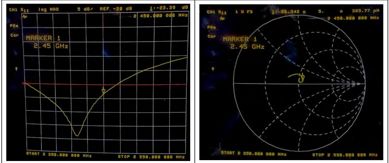
Dipole Verification Data
